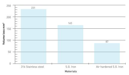
The actual wear rates can vary from the laboratory results nominated. They can be effected by such things as wet service, particle size, cavitation and impingement angle.
