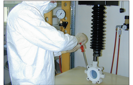
Valve assembly in clean room
